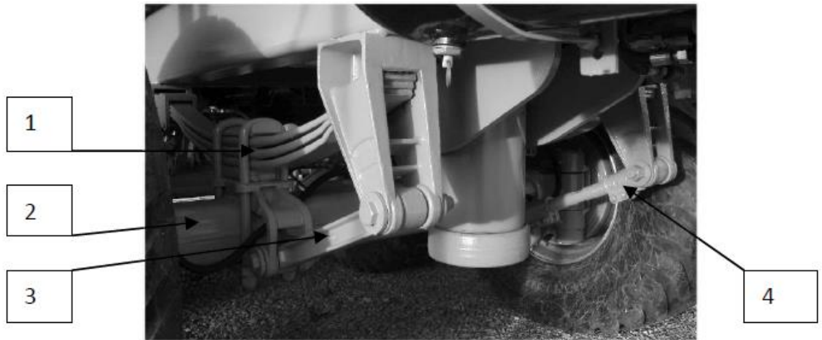
Fig. 7.13. Diagram of the installation of the axle. 1 – springs; 2 – axle; 3 – non-adjustment rod; 4 – adjustment rod.
