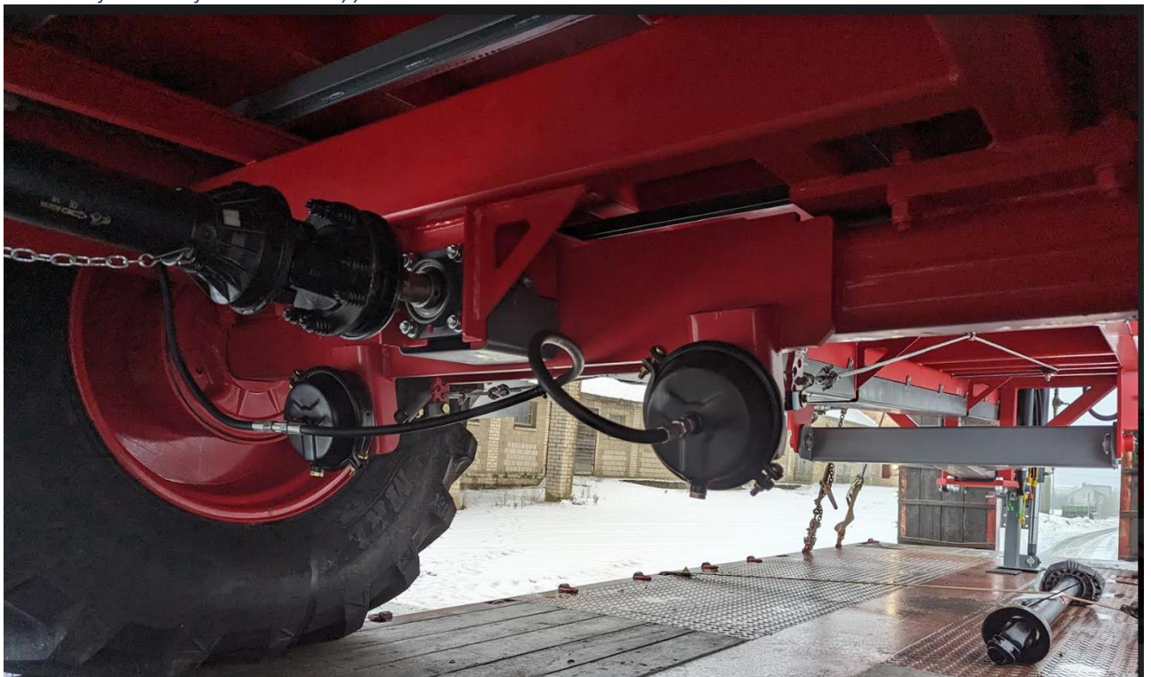
4.5 pav. Bypass clutch; friction clutch.
