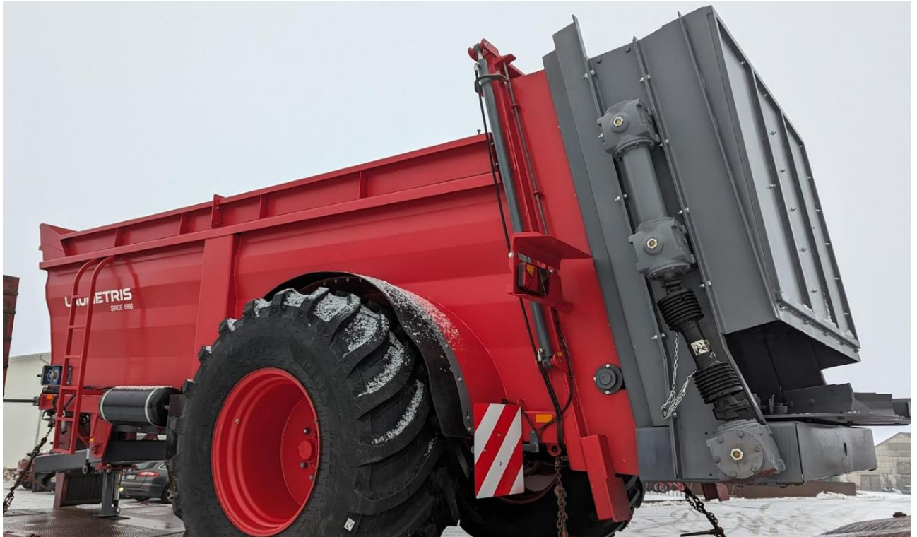
Fig. 4.4 Horizontal manure spreader gears; Spreader transmission pto shaft; spreader transmission gear (comes fully assembled from manufacturer – Berma.)
